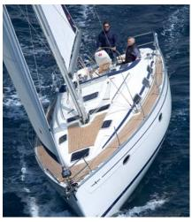
Slx opening hatches and two non-opening deck skylights for a brighter interior and better ventilation
